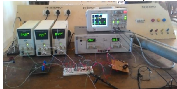
Fig.17 (c) Proposed Converter with DC Load as Resistor (another view of overall system)
