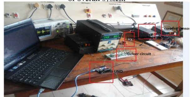
Fig 17 (a) Laboratory experimental setup for testing the FL MPPT controller using Arduino UNO with proposed KY – SR Buck Boost converter
