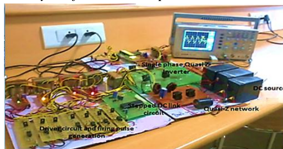
Fig. 10. Experimental setup of single phase seven level SDCqZSI inverter
