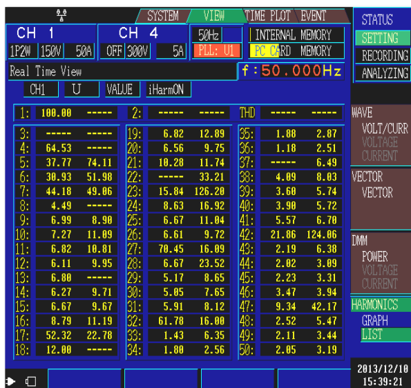
Figure 17 THD Analysis for 5-Level inverter.
