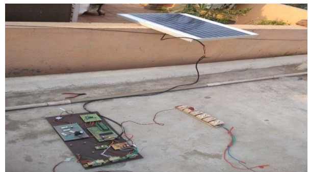
Fig.15 Experimental setup of boost converter connected with 37W solar panel
