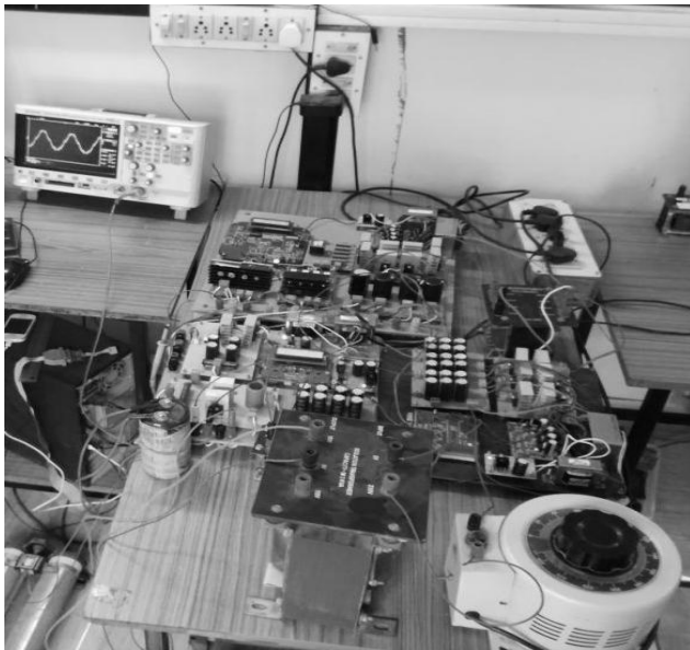
Fig. 16.c. Hardware implementation of 15level MLI with single input triple output DC-DC boost converter
